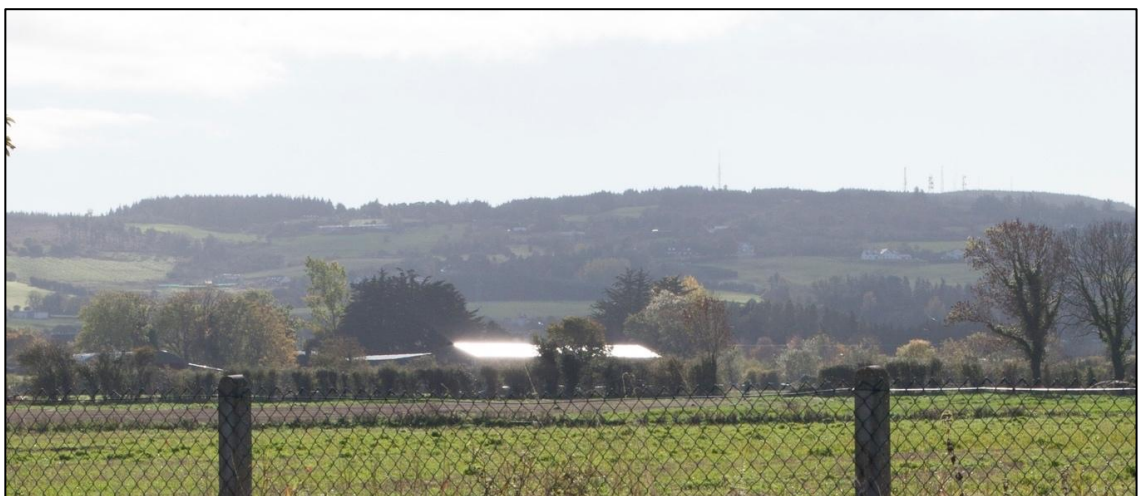
Figure 1.5: Higher levels of reflectance (to photovoltaic panels) emanating from powder coated corrugated metal roof surfaces in an Irish rural scenario.
